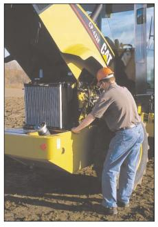
The one-piece fiberglass hood tilts for exceptional access to the engine and cooling system. Daily service points are accessible from ground level and are grouped on one side of the engine.
