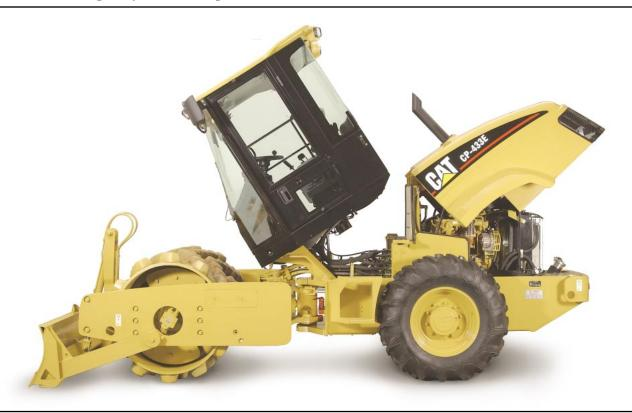
**Visual indicators** allows easy check of radiator coolant, hydraulic oil tank level and air restriction indicator.
