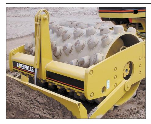
The padfoot drum has 108 pads welded on the drum in a chevron arrangement.
