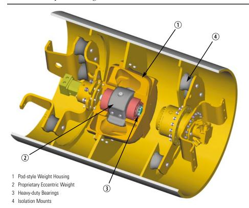
**Pod-style weight housing** is assembled and sealed at the factory to ensure cleanliness, longer bearing life and easier field exchange or service.
