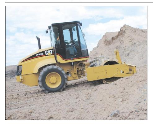
**Two propel pump system** has dedicated pumps to drive the heavy-duty, hightorque rear wheel and drum motors independently. Should the drum or wheels begin to spin, there is always hydraulic flow to the non-spinning motor, allowing continuous tractive effort. Especially useful in loose underfoot conditions.
