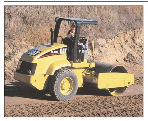
**Visibility** to the tire edges and rear of machine is exceptional. The sloped hood allows the operator to see obstacles measuring 1 meter (3' 3") high located 1 meter (3' 3") to the rear of the machine. Excellent visibility increases productivity when working near obstructions or maneuvering around the job site.
