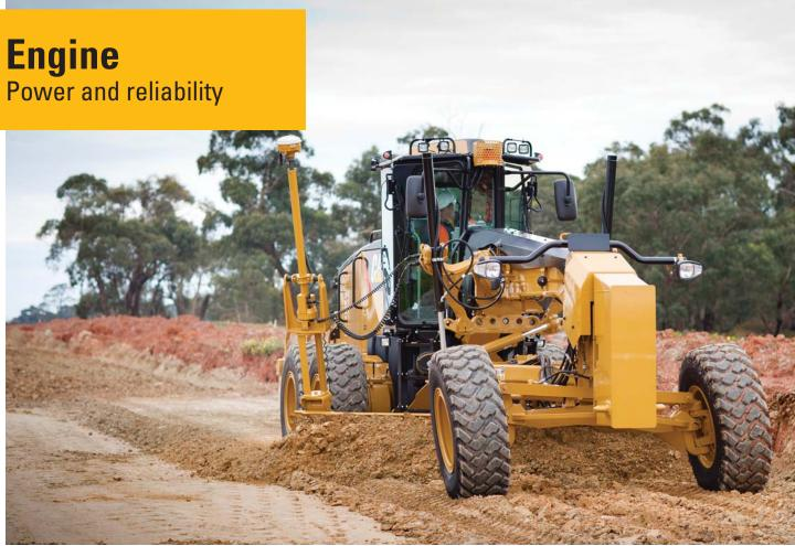
Cat C7 and C9 ACERT engines give you the performance you need to maintain consistent grading speeds for maximum productivity. Superior torque and lugging capability provide the power to pull through sudden, short-term increases in loads.
